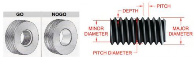
Fig. 4 — If the 2A NOGO gage goes over, then the threads are nonconforming according to ASME B1.3 System 21.
